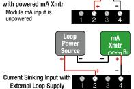
Customer-supplied external contacts for **Output Test Function** Switch closure sets output to approx. 50% of span
