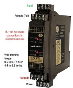
\* To avoid damage to the module, do not leave any unused mA outputs disconnected. Use a 1000 0hm 1/2 Watt resistor across terminals 9 & 10 or 11 & 12 if any are not being used.
