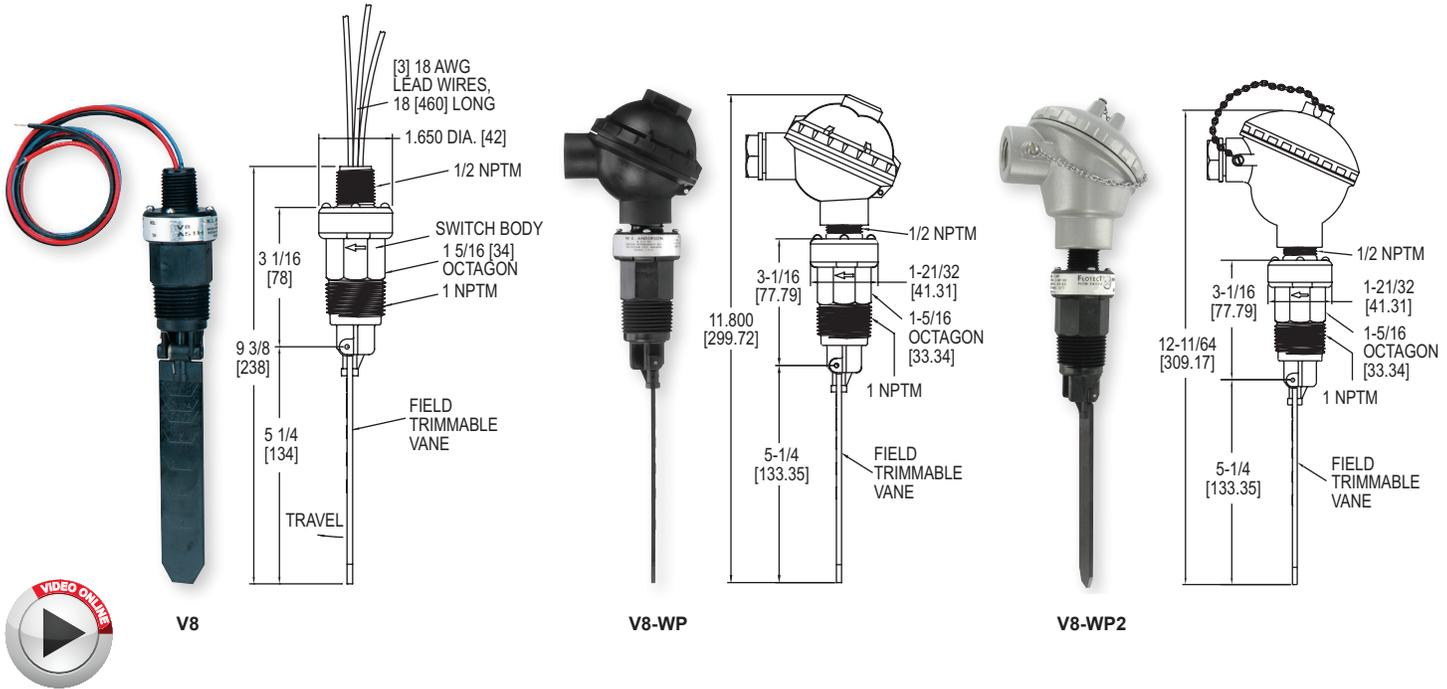
The **Series V8 Flotect® Vane Operated Flow Switches** are ideal for protecting unattended equipment from damage or loss of production. This Series is available for installation in a 1 to 6" pipe with operating pressures up to 150 psig (10 bar) and temperatures to 212°F (100°C).
