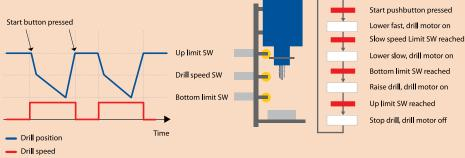
Bottom limit SW reached Raise drill, drill motor on Up limit SW reached Stop drill, drill motor off
