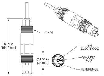
AquaSensors AnalogPlus Differential pH Sensor - 1.0 in.
