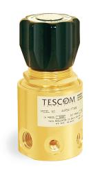
TESCOM 44-1500 Series high flow/low pressure regulator controls outlet pressures up to 600 psig / 41 bar. Large area piston provides accurate pressure control and cycle life superior to diaphragm sensed regulators when applied to heavy duty cycling. Features a segregated/captured vent for hydraulic or pneumatic media and is available in two outlet spring ranges. Optional dome or air loaded versions for remote operation or for use with the TESCOM ER5000 Electropneumatic Controller for automation.
