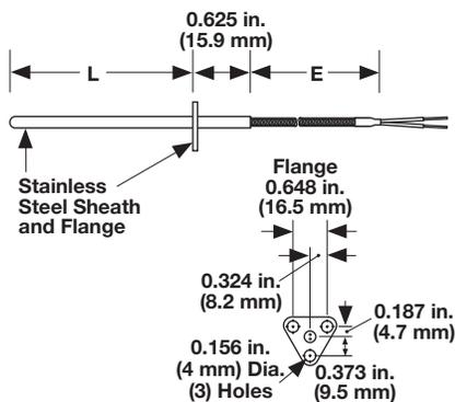
The flanged thermocouple allows rapid assembly and low profile when going through bulkheads.
