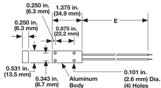
Low profile aluminum block for fast accurate surface measurement.
