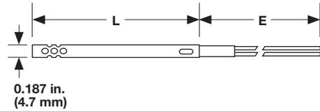
Aspirated tube design allows air to flow directly over thermistor for fast time response.
