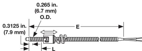
Adjustable armor thermocouples bend to any angle to fit a wide range of hole depths, eliminating the need to stock numerous styles. A stainless steel hose offers additional lead protection in demanding applications.
