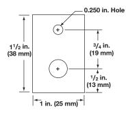
A 1% in. (38 mm) x 1 in. (25 mm) wide x 16 gauge stainless steel bracket with one element hole and one mounting hole % in. (13 mm) from end.
