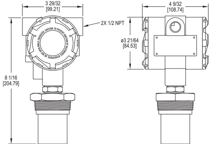
The **Series ULT Ultrasonic Level Transmitter** provides non-contact measurement of liquid levels in an explosion-proof body. It is capable of measuring up to 32.8' (10 m) with a PVDF sensor and 4-20 mA output.
