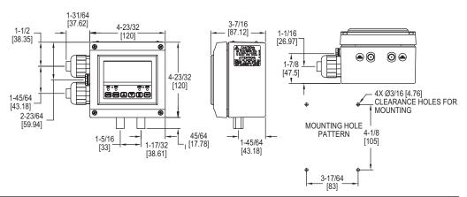
The Series DHII Digihelic® II Differential Pressure Controller takes all the features of the standard Digihelic® pressure controller and packages them in a robust NEMA 4 (IP66) housing.
