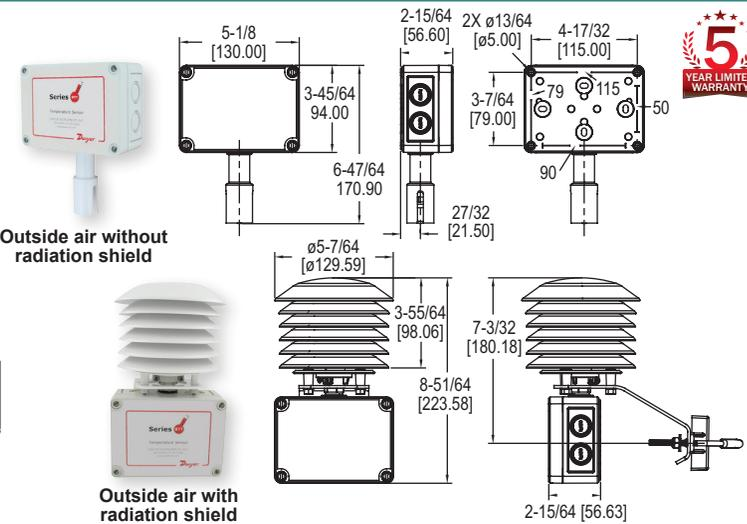
The **Series BTT Temperature Transmitters** offer transmitter output signals with the same form and fit as our popular TE thermistor and RTD sensors for building HVAC applications. Thermowells are required when using immersion models in liquid applications.
