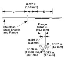
The flanged thermocouple allows rapid assembly and low profile when going through bulkheads.
