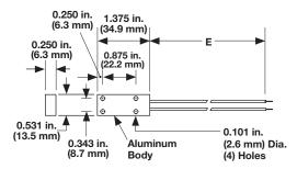
Low profile aluminum block for fast accurate surface measurement.
