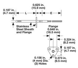
Aspirated tube design allows air to flow directly over thermistor for fast time response with a flange for mounting sensor.
