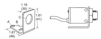
**Hole center spacing:** A to B = 0.95 (24.2) **Hole size:**
