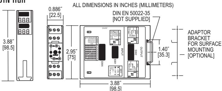
The **Series SC1 Process/Temperature Alarm Switch Module** is an on-off or limit switch with selectable process signal. Each unit has two form C (SPDT) relays which can operate independently, or be logically connected to operate as a DPDT output.
